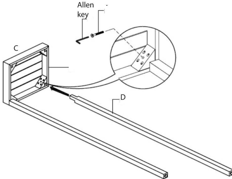
2. Insert the 4 Shelves (E) into the opening between the two previously-installed legs, align the holes from the leg with the corresponding holes on the center of the shelf bracing (located on each corner). Apply bolt (B) into the center hole of the shelf bracing as shown. Tighten fully using the enclosed Allen key.
