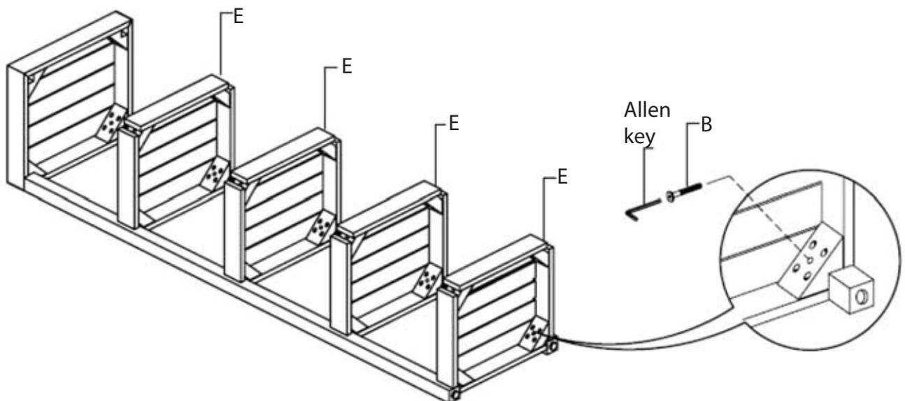
3. Insert the remaining legs (D) into the openings located at each corner of the top (C). Once the leg is fully inserted, apply bolt (A) into the center hole of the top bracing as shown. Tighten fully using the enclosed allen key. Align the holes from the leg with the corresponding holes on the center of the shelf bracing (located on each corner). Apply bolt (B) into the center hole of the shelf bracing as shown. Tighten fully using the enclosed allen key.
