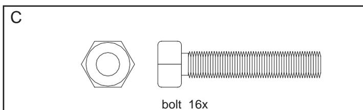
1. Carefully flip table top over and lay onto scratch-free surface such as carpet or cardboard. Align leg with holes on table top as drawing shows. Insert bolt (C), lock washer (B), and flat washer (A) into hole and tighten with supplied wrench. Once all four legs are installed flip the table over (This will require the help of another person). Levelers may need to be adjusted to accommodate uneven floors.
