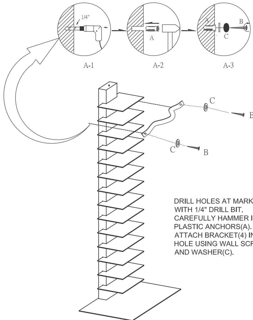
DRILL HOLES AT MARKED SPOTS WITH 1/4" DRILL BIT.
