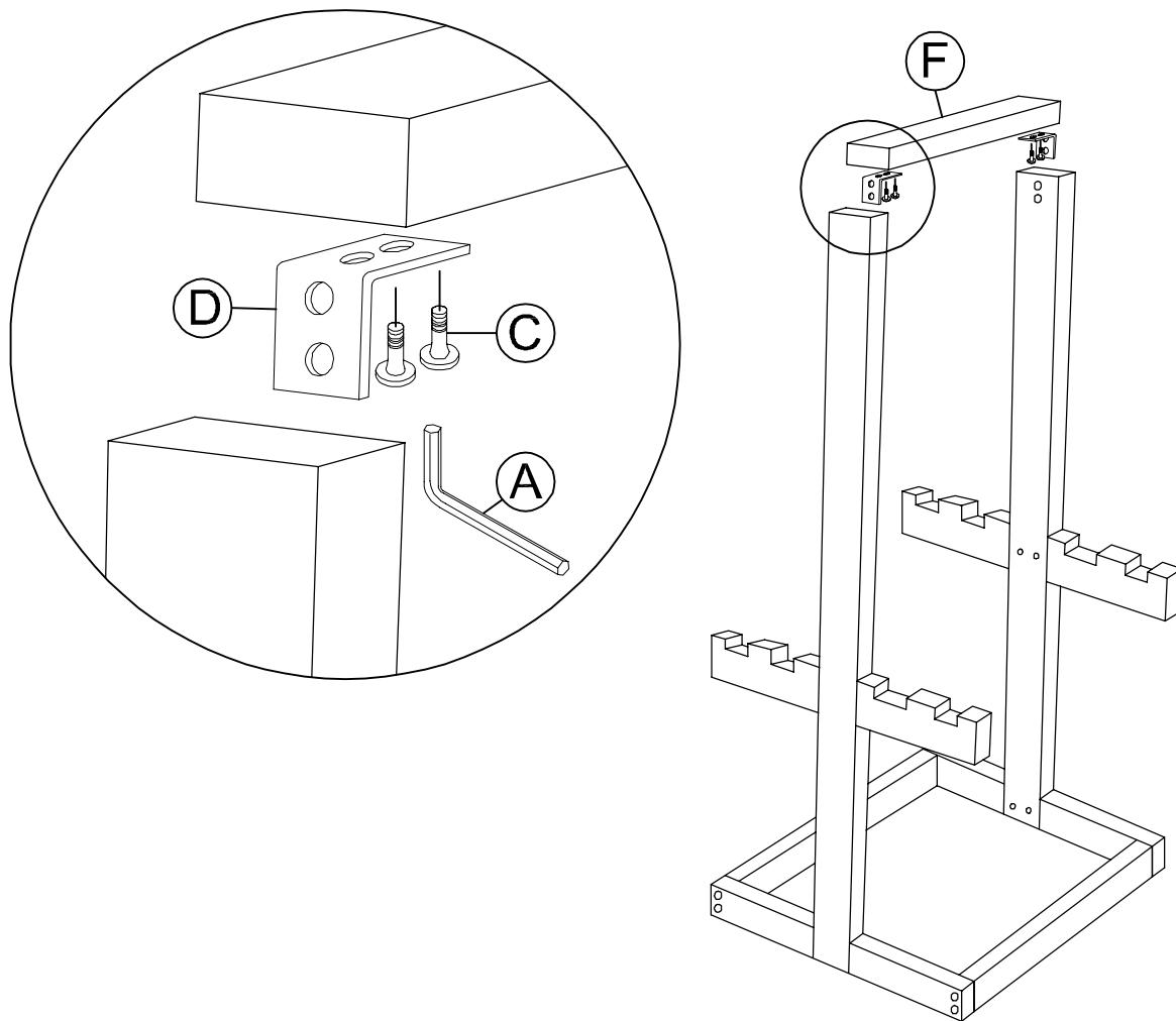
3. Insert bolts (C) into brackets as shown. Tighten with supplied hex key (A).
