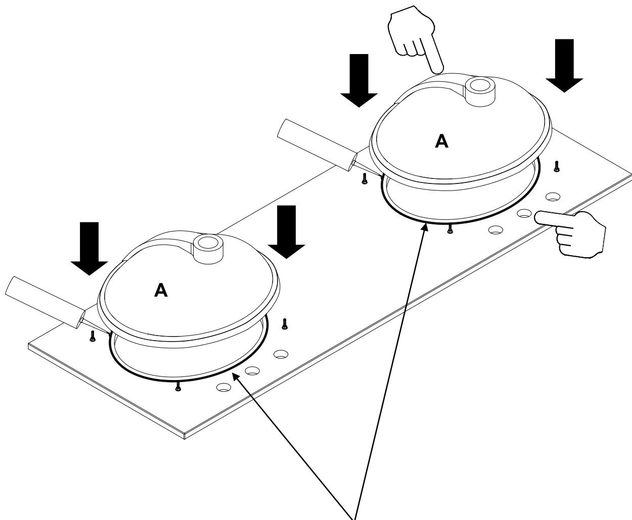
To Seal The Connection Between The Basin Edge And The Bottom Of The Stone Top.
