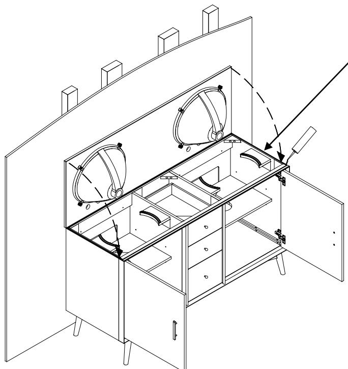
To Seal The Connection Between The Bottom Of The Stone Top And The Top Of The Wood Vanity Top.
