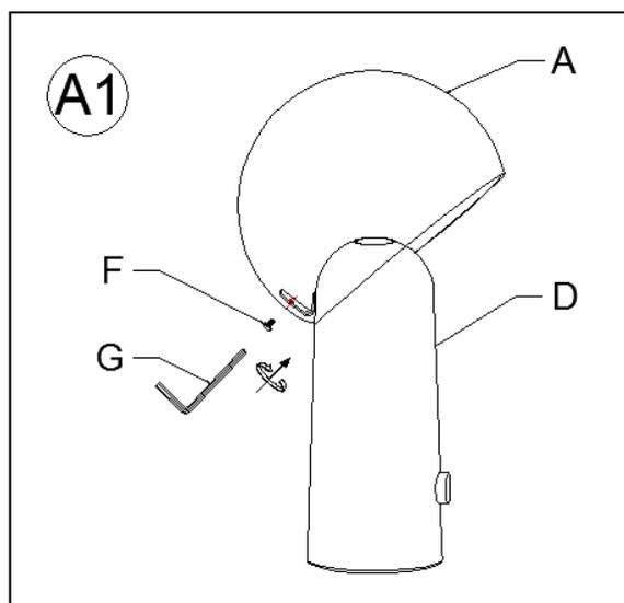
1. Attach the Shade (A) onto the bracket of Base (D), making sure the screw holes on both parts are aligned. Insert the Screw (F) and fasten with an Allen Key (G). Rotate screw clockwise until tight.
