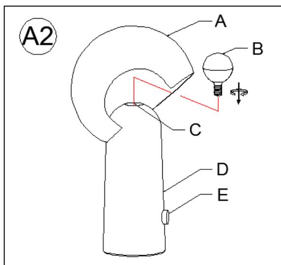
2. Insert the specified light bulb into the Socket (C). DO NOT EXCEED THE SPECIFIED WATTAGE.
