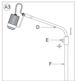
If needed, loosen the Clamping Nut (E) by turning anticlockwise.
