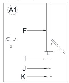
1. Unscrew the Nut (K), Toothed Washer (J) and Flat Washer (I) from the bottom of Lower Tube (F) by turning counter-clockwise.
