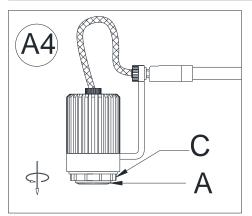
4. Unscrew the Socket Ring (C) from the Socket (A) by rotating counter-clockwise.
