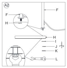
Insert the bottom threaded portion of Lower Tube (F) through the hole on the Base (H). Position Flat Washer (I), Toothed Washer (J) onto the protruded threaded portion of Lower Tube (F). Secure using the Nut (K) and tight firmly with a Wrench (L) provided.
