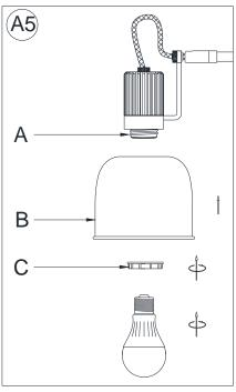
Attach the Shade (B) onto the Socket (A). Secure Shade
