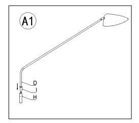
1. Insert the Joint (I) into the Low Stem (H), aligning the holes in the Joint (I) with the holes from the Low Stem (H).
