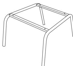
1. Lay the chair back onto a clean smooth surface such as carpet or cardboard. Align base. Insert bolt (A), lock washer (C), flat washer (B). Tighten with supplied hex key (E). Cover bolts with plastic caps (C).
