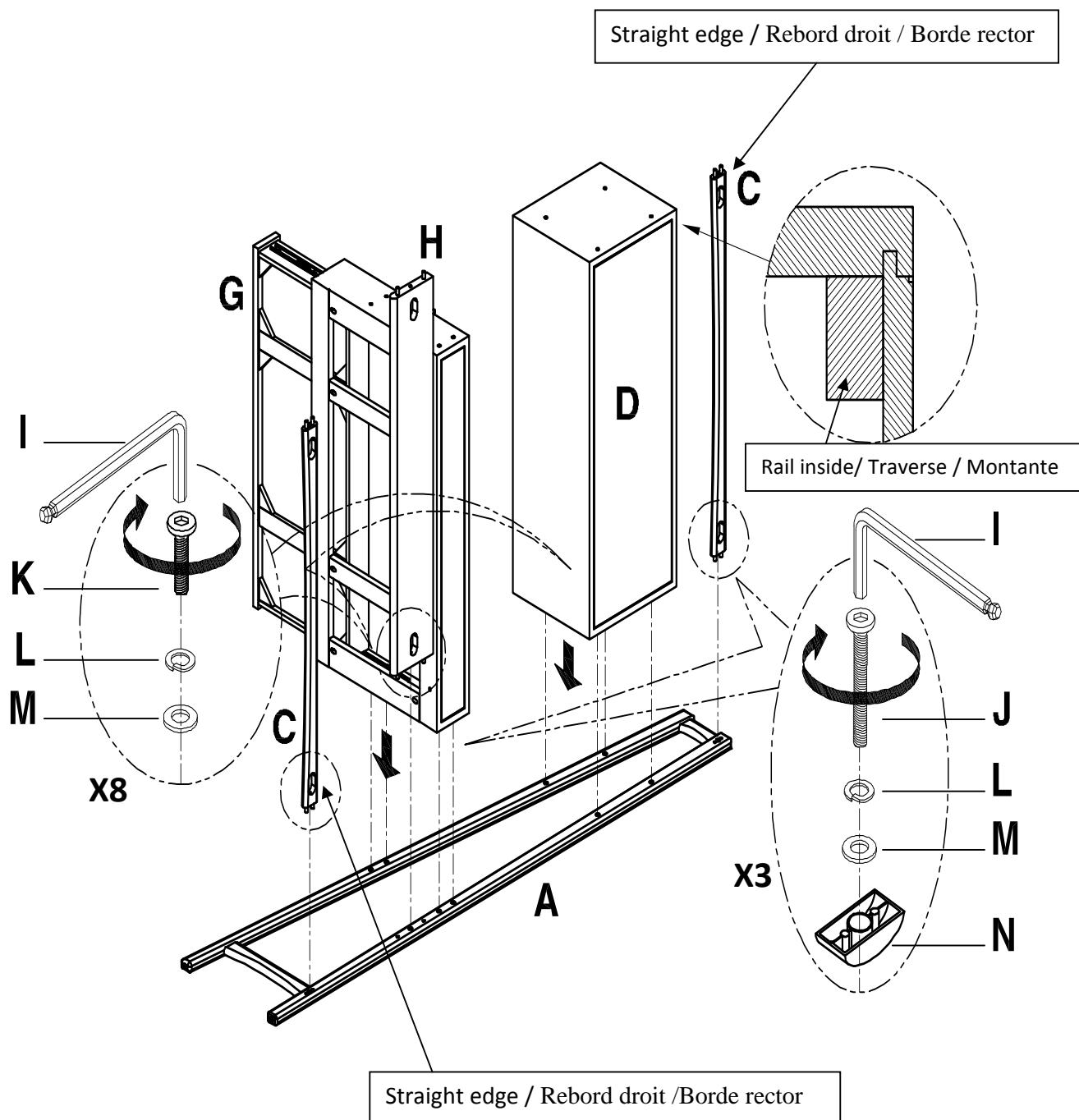
5. - Attach the Right Leg Frame (B) onto the assembled piece ad repeat the previous steps to connect. Check alignments before tightening.
