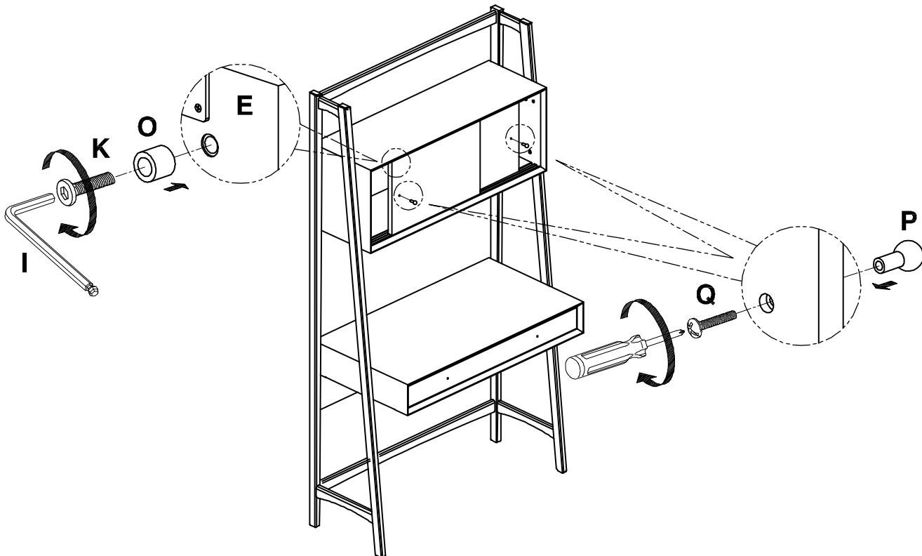
12. - Attach Pulls (P) to pre-drilled holes on the drawer front and insert Machine Screws (Q) from the other side to secure. Do not over tighten.
