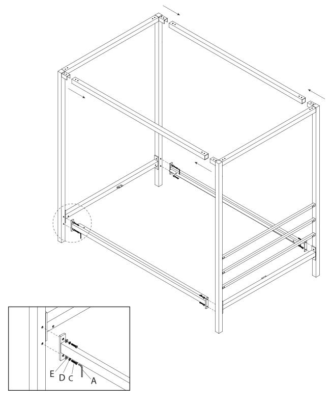
4. Fasten top rails to uprights using socket screws (B). Tighten using allen key (A).
