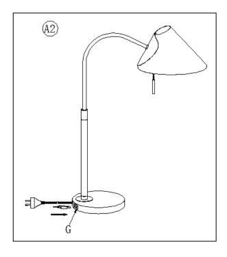
There is one USB Port (G) on the lamp base, which can be used for recharging USB devices (USB charging cable is not included). **The maximum output is DC 5V, 2A.** Do not overcharge.
