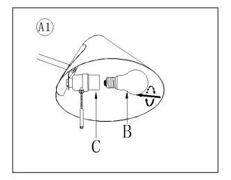
Insert the specified light bulb into the Socket (C).
