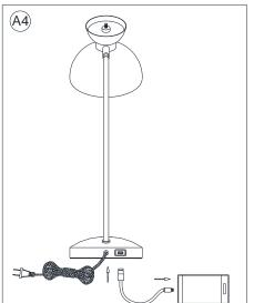
5. Plug the power cord into the proper electrical outlet and test fixture.
