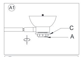
1. Unscrew the Socket Ring (C) from the Socket (A) by rotating counter-clockwise.
