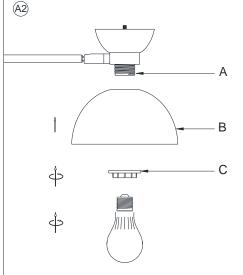
2. Attach the Glass Shade (B) onto the Socket (A). Secure Glass Shade (B) by rotating the Socket Ring (C) onto the Socket (A) in a clockwise direction until tight.
