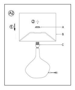
Place the Shade (B) over onto the Socket (C) and secure the shade in place by turning the Socket Ring (A) in a clockwise direction until tight.
