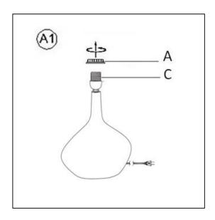
Unscrew Socket Ring (A) from Socket (C) by turning counter-clockwise.
