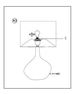
Insert the specified light bulb into the Socket (C). DO NOT EXCEED THE SPECIFIED WATTAGE.
