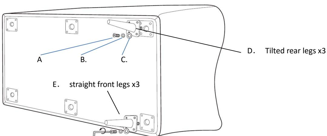
Each leg will have 4xbolts w/lock washer and flat washer to fix
