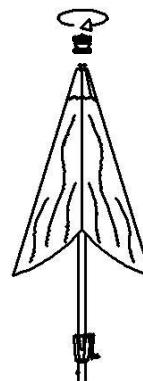
2. Secure lower pole into upper pole and lock into place. Secure the umbrella into the umbrella stand. Tighten the knobs on the base to secure the umbrella to the base.
