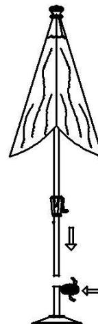
3. To open the umbrella, wind the crank handle clockwise until the runner reaches the stopper ring. To tilt the umbrella simply continue to crank and upper portion will automatically tilt.
