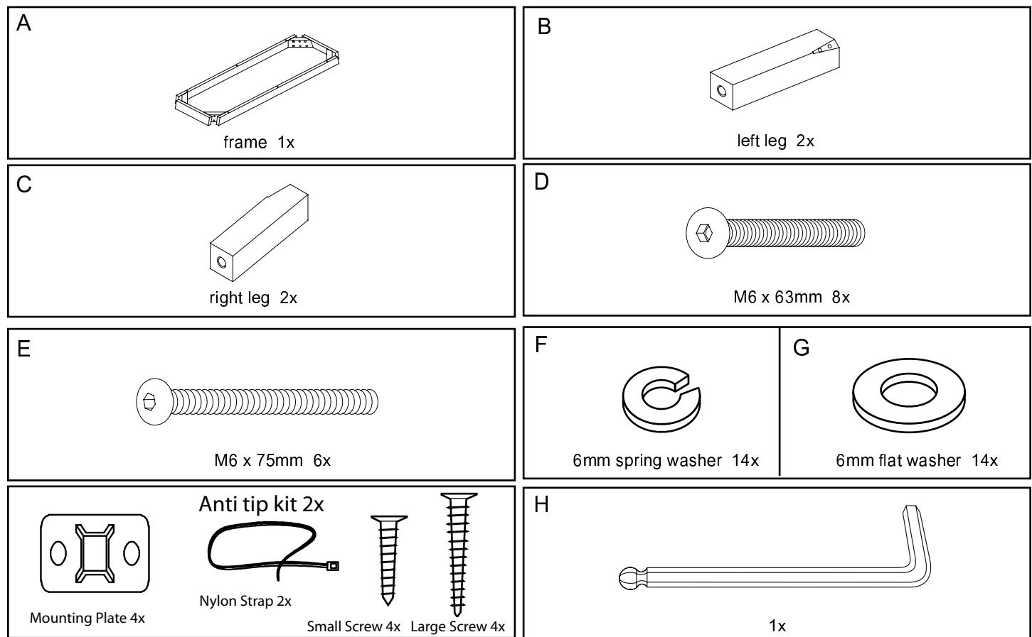
1. Align legs as shown, Insert bolt (D), lock washer (F), and flat washer (G). Tighten with supplied hex key (H).
