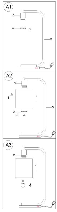
1. Unscrew the Socket Ring (A) from the Socket (C).
