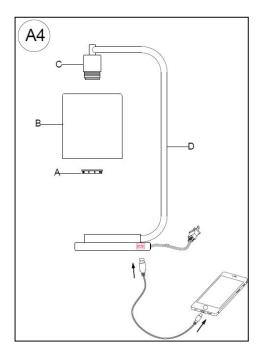
If needed, gently and appropriately insert the USB devices on the side of lamp base until secure.
