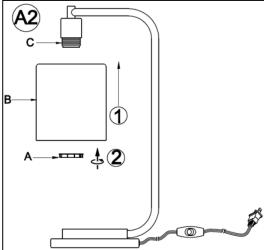
2. Place the Glass Shade (B) onto Socket (C). Secure the Glass Shade (B) in place by turning the Socket Ring (B) in a clockwise direction until tight.
