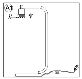
1. Unscrew the Socket Ring (A) from the Socket (C).
