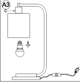
3. Insert the specified light bulb into the Socket (C). DO NOT EXCEED THE SPECIFIED WATTAGE.
