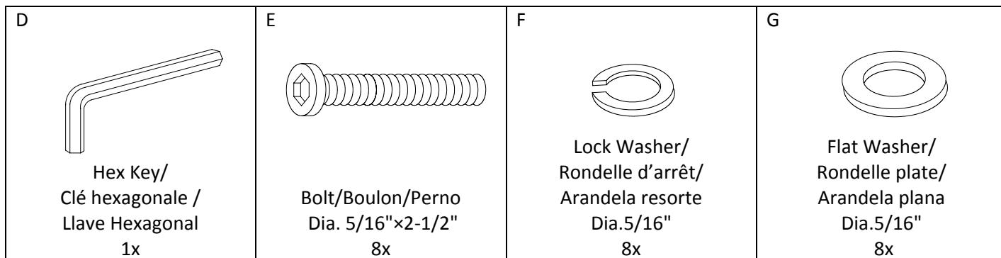
1. Lay table top upside down on a clean smooth surface such as carpet or cardboard. Align legs with bottom of table as shown. Insert bolt (E), lock washer (F), and flat washer (G) through holes in corner blocks and into legs. Tighten with hex key (D). Repeat this step for other legs.
