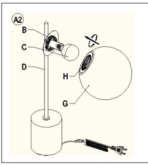
2. Attached Shade Inner Thread-Ring (H) onto the Shade Outer Thread-Ring (B), then turning Glass Shade (G) in a clockwise direction until tight. Please don't over tight.
