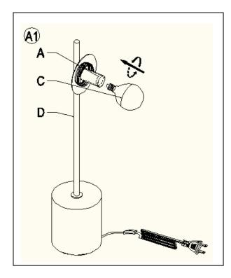
Insert the specified light bulb into the Socket (A). DO NOT EXCEED THE SPECIFIED WATTAGE.
