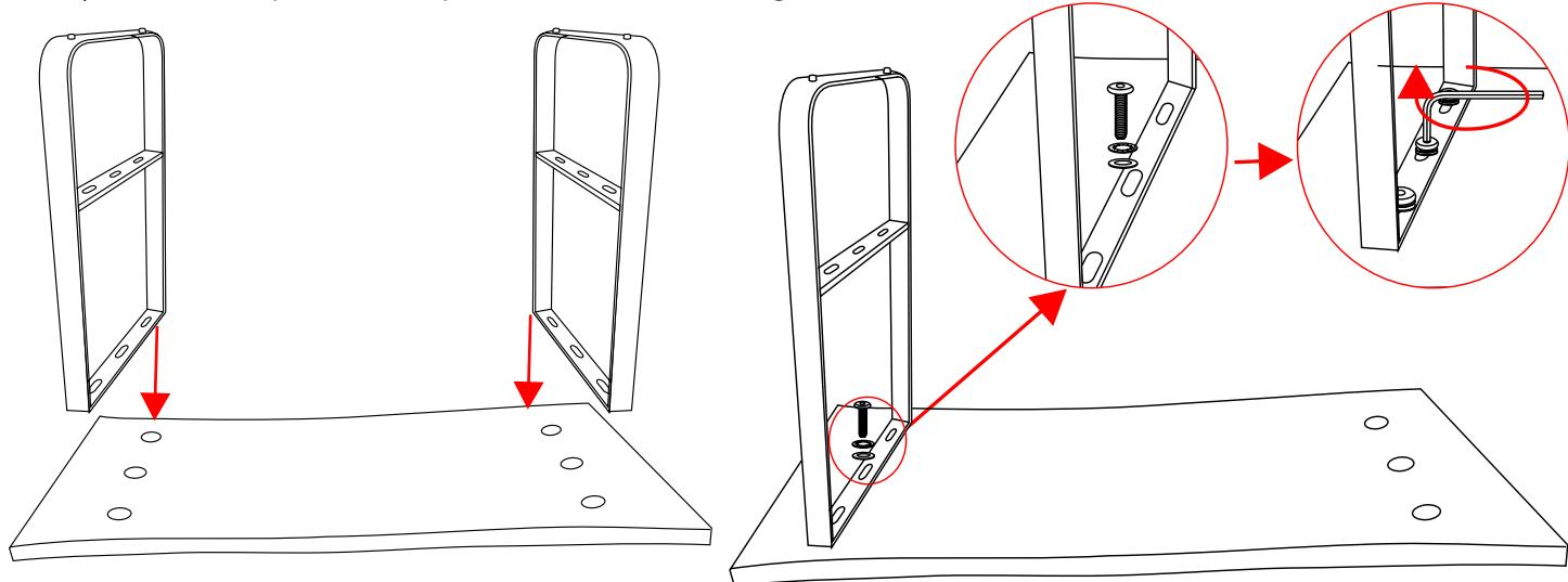
2. Align shelf with the legs as shown. Insert bolts (A). Tighten with supplied hex key (D).
