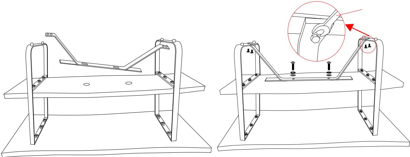
4. Insert adjustable levelers (C). Tighten by hand. These may need to be adjusted to accomodate uneven flooring.
