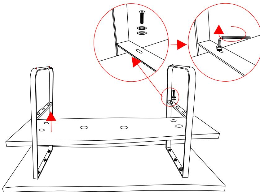
3. Align center bracket with legs as shown. Insert bolt (B). Tighten with wrench (Not supplied).
