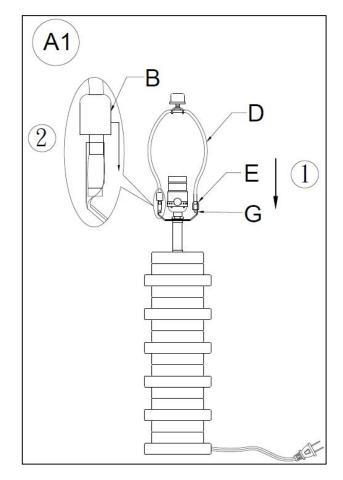
1. Raise the Harp Caps (E) and insert the bottom ends of Harp (D) into the Saddle (G). Lower the Harp Caps (E) until they cover the two-pronged Saddle (G).
