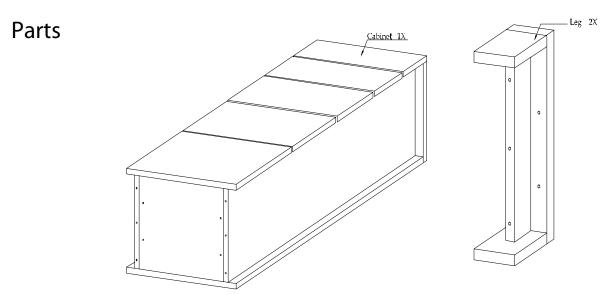
1. Carefully lay the case back on a soft surface, such as: cardboard or carpet to protect finish. Assemble leg on cabinet with 3 bolts (B), 2 bolts (A) with lock washers (C) as shown below.
