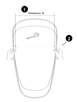
3. Connect the two marks of Step (2) with a light pencil line and use a level to ensure the line is level. Make two "insertion marks" centered along this line with a measurement equal to "Distance A".
