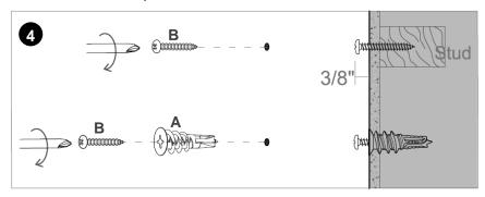
How to install the anchor? Place a Phillips screwdriver into the recess of the anchor and firmly press
