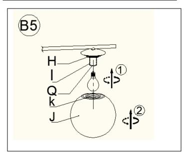
5. Insert the specified light bulbs into the Sockets (Q). DO NOT EXCEED THE SPECIFIED WATTAGE. Hold the glass shades (J) and attached Shade Inner Thread-Rings (K) onto the Shade Outer Thread-Rings (H), then turning in a clockwise direction until tight.
