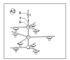
2. If you would like to use only one 12 in. Tube (E), then thread the 2 wire power cords through the 12 Inch Lamp Tube (E), making sure the tube nipple joint end is downward as shown in diagram A2. Attach the bottom end of 12 Inch Lamp Tube (E) onto the top end of 6 in. Tube (F) and rotate clockwise until tight.
