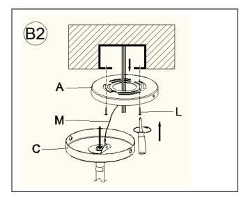
2. Insert the J-box wires through the center opening of the Mounting Plate (A). Attach the Mounting Plate (A) to the junction box using the two J-Box Mounting Screws (L). Tighten each screw clockwise until the Mounting Plate (A) is firmly secured to the J-Box. Then the steel wire (M) can hang up the fixture securely.
