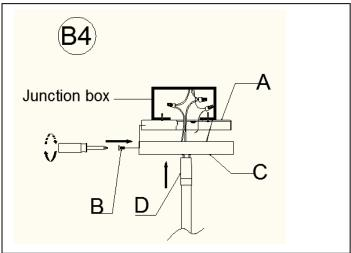
4. With the help of another people to hold the weight of the light fixture, Raise the Canopy (C) up over the Mounting Plate (A). Align the holes on the Mounting Plate (A) with the holes on the side of the Canopy (C). Insert the 3 Canopy Screws (B) and tighten with a screwdriver.
