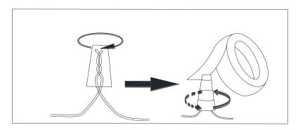
Connect the GROUND FIXTURE WIRE to the GROUND J-BOX WIRE using the Plastic Wire Nut Connector (N) and wrap the connection with electrical tape. Be sure that no wire strands are exposed.
