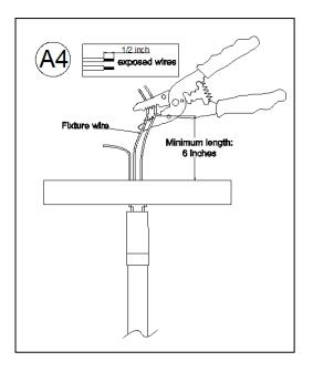
If needed, cut off the extra power cord length on the 2 wires so that they are at least 6 inches (152.4 mm) long within the outlet junction box (J-box).
