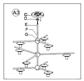
3. Use the additional 12 Inch Lamp Tube (E) as needed to adjust the fixture's suspension length by following the similar procedure as outlined in step 2. Once the fixture's suspension length is determined, thread the 2 wire power cords through Ball Joint (D) and Canopy (C). Attached the Ball Joint (D) onto the 12 Inch Lamp Tube (E) and rotate clockwise until tight.
