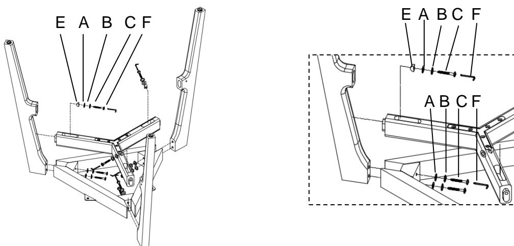
2. Lay the TABLE TOP onto a clean smooth surface such as carpet or cardboard. Align legs as shown. Insert bolt (D). Tighten with Allen key (F). If the floor is uneven, adjust the glider on the bottom of the Leg.
