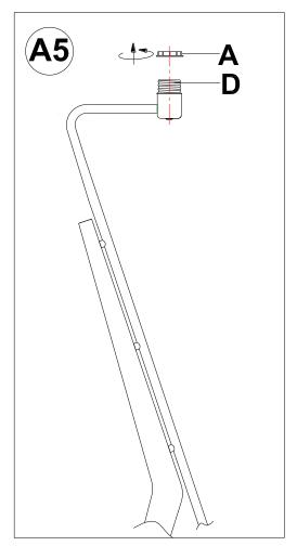
Unscrew Socket Ring (A) from Socket (D) by turning counter-clockwise.
