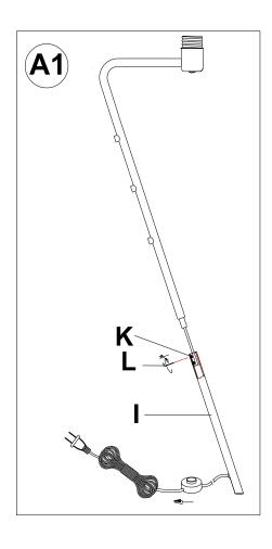
1. Loosen the Set Screws (K) from the Lower Tube (I) using the Allen Key (L) by turning Set Screws (K) in a counter-clockwise
