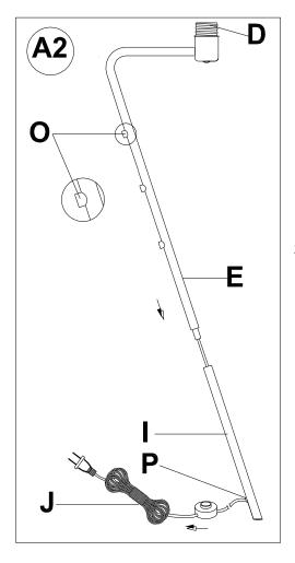
2. Insert the Top Curved Tube (E) into the Lower Tube(I), align short screw tubes (O) with Exit Hole (P) in the same line.
