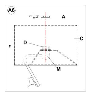
Place the Shade (C) onto the Socket (D), Secure the Shade
