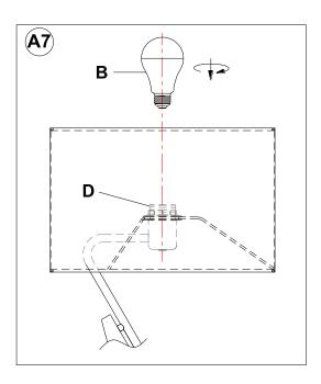
7. Insert the specified light bulb (B) into the Socket (D). DO NOT EXCEED THE SPECIFIED WATTAGE.
