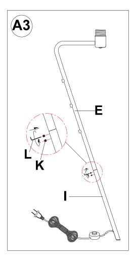
Secure the Set Screws (K) onto on the Upper Curved Tube (E) using the Allen Key (L) until tight.
