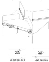
**Step 11: Assemble Modesty Screens.** Align Screen hook with Toolbar. Repeat 4 times. Assembly complete.
