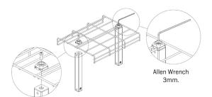
**Step 9: Attach Wirebaskets.** Align Wirebasket assembly with pins on the underside of the Toolbar then tighten set screws. Repeat 4 times.
