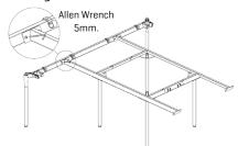
**Step 5:** Assemble outside rails to outside legs both sides and tighten set screws.
