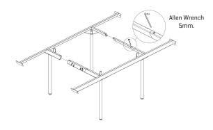
**Step 3:** Assemble 2 outside leg assemblies. Make sure to use circlet rails. [2 Sets]
