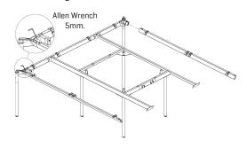
**Step 6:** Assemble the 2<sup>nd</sup> leg assembly to complete Frame. Tighten set screws using enclosed M8 SHCS to attach H Frame. Frame complete.
