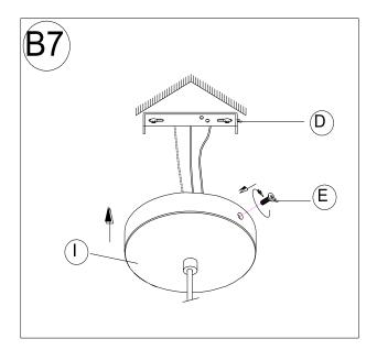
7. With the help of another person to hold the weight of the light fixture, position the Canopy (I) over the Mounting Plate (D), aligning the 2 holes on the Canopy (I) with the 2 holes from the Mounting Plate (D). Insert the 2 Canopy Screws (E) and tighten to secure the Canopy (I) in place.
