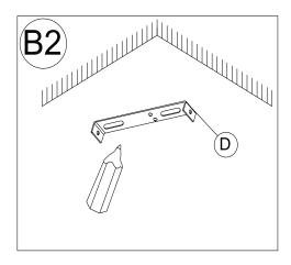
2. Determine the desired location for the light fixture, place the Mounting Plate (D) against the ceiling and mark the location of the slots of Mounting Plate (D) onto the ceiling using a pencil.
