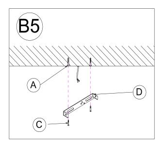
Attach the Mounting Plate (D) onto the ceiling aligning the 2 slots on the Mounting Plate (D) with the installed Plastic Anchors (A). secure the mounting plate (D) by Inserting each Mounting Screws (C), turning each Mounting Screw (D) in a clockwise direction with a screwdriver until tight.
