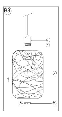
8. Attached shade onto the Socket (K), Secure shade by tightening the Socket Ring (M) in a clockwise direction until tighten.
