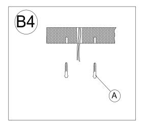
Insert each Plastic Anchors (A) into each Drilled hole on ceiling.
