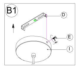
1. Separate the Mounting Plate (D) from Canopy (I) by removing the Canopy Screws (E). Do not discard the Canopy Screws (E) as these will be used later.
