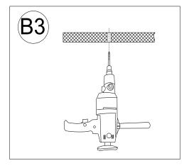
3. Using the drill with the appropriate size drill bit (just large enough to make hole that will allow passage of the Plastic Anchors (A) assemblies), drill one hole in the ceiling at each marked slot location for the Plastic Anchors (A).
