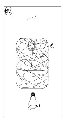
Insert the specified light bulb into the Socket (K). DO NOT EXCEED THE SPECIFIED WATTAGE.
