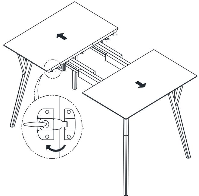
3. Carefully align the extension as shown. Align the pins on the extension with the pin holes on the top. With one person on each end press the table together and lock the table locks by turning the counterclockwise.
