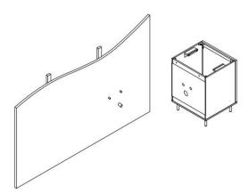
Install proper mounting hardware in wall. Attach vanity to wall.
