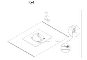
Hand tighten with wrench till Basin does not move. Over tightening can cause damage. Let Sealant cure according to manufacturer's directions before installing on vanity case.
