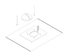
Place Basin on Marble Top. Basin drain is towards the faucet holes. Wipe off excess Sealant **F** (Hold Down)
