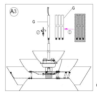
3. Take out 3 Long Tubes (G) from poly bag. If you would like use only one Long Tube (G), the thread the power cord through it, make sure the tube nipple joint end is downward. Attach the Long Tube (G) onto the top of Short Tube (H) and rotate Long Tube (G) in clockwise direction until tight.
