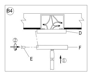
4. With the help of another person to hold the weight of the light fixture, position the Canopy (F) over the Mounting Plate (D), aligning the 3 holes on the Canopy (F) with the 3 holes from the Mounting Plate (D). Insert the 3 Canopy Screws (E) and tighten to secure the Canopy (F) in place.
