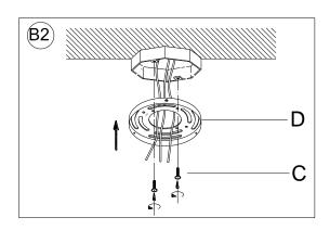
2. Gently pull existing wire down from the ceiling junction box and allow wires to hang. Attach Mounting Plate (D) to the ceiling outlet box, aligning the slots of the Mounting Plate (D) with the two threaded holes located on the J-Box. Insert and tighten 2 Mounting Screws (C) with a screwdriver.
