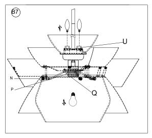
7. Insert the specified light bulbs into the Sockets (Q&U). DO NOT EXCEED THE SPECIFIED WATTAGE.
