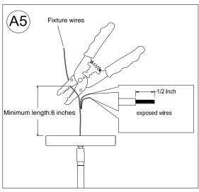
If needed, cut off the extra fixture 3 wire power cord length so that they all are at least 6 inches (152.4 mm) long within the outlet junction box (J-box)
