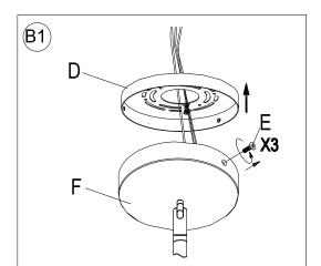
Separate the Mounting Plate (D) from Canopy (F) by removing the Canopy Screws (E). Do not discard the Canopy Screws (E) as these will be used later.
