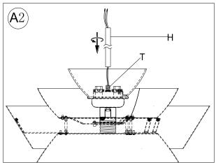
2. Insert the fixture wire through the Short Tube (H), and attach the Short Tube (H) onto the Threaded Pipe (T) and turning Short Tube (H) in clockwise direction until tight.
