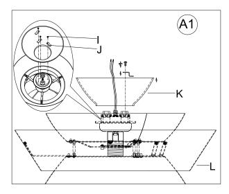
Attach the Top Glass Shade (K) onto the Top Housing cover (S), Place "Z' Metal sheets (J) onto the Top Glass Shade (K), Secure the Top Glass Shade (K) by tightening the "Z' Metal sheets (J) using the Set Screws (I). Make sure the "Z' Metal sheets (J) and Top Glass Shade (K) are fixed together and security. Please don't over tighten the Set Screw (I).
