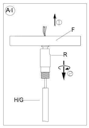
Thread the fixture 3 wire power cord through the Ball Joint (R) and Canopy (F).
