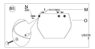
Position the Metal Bracket into the Bottom Glass Shade (O), Align holes of the Bottom Glass Shade with the Screw Holes at the end of spiders of the Metal Bracket (M), Insert the 3 Thumb Screws (N) and tighten in a clockwise. Please don't over tighten.
