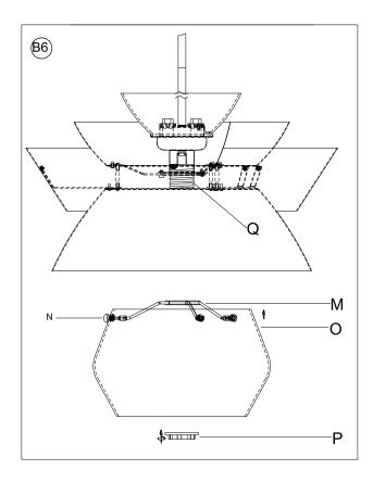
Attach assembled Bottom Glass Shade (O) and Metal Bracket (M) onto Socket (Q). Secure assembled Bottom Glass Shade (O) and Metal Bracket (M) by turning the Socket Ring (P) in clockwise direction until tight.
