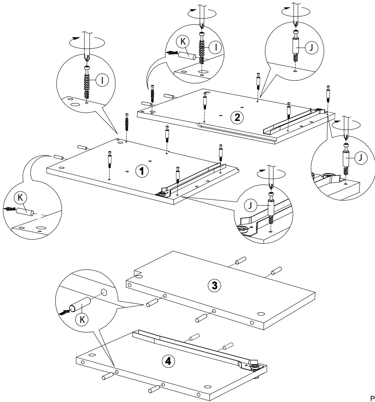
8. Insert large dowels (K) into back rail.
