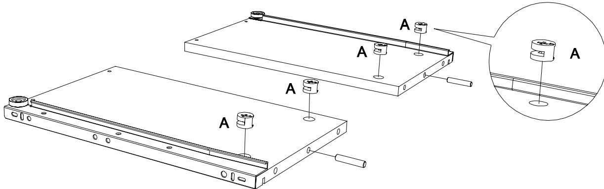
2. Insert small cam bolts (B) into drawer front like the drawing shows.
