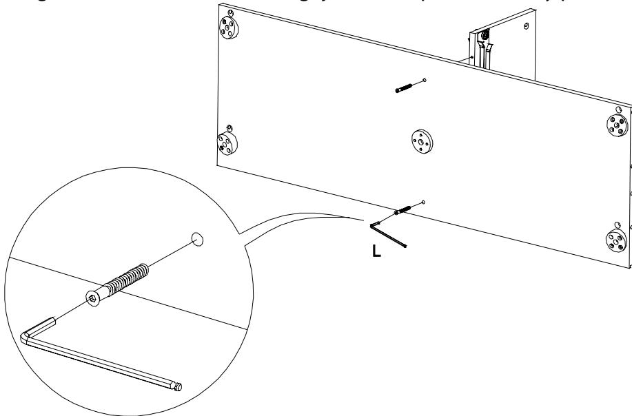
11. Insert 2 connecting bolts (L) thru shelf into partition A. Tighten with supplied allen key.
