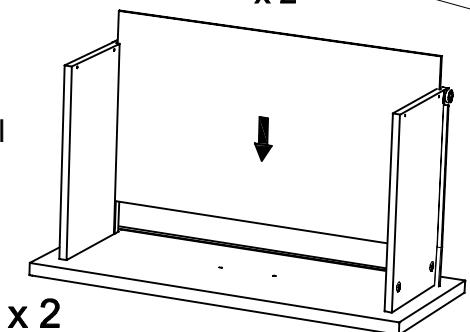
5. Attach drawer back to drawer sides. Insert large screws (D). Tighten with screw driver.
