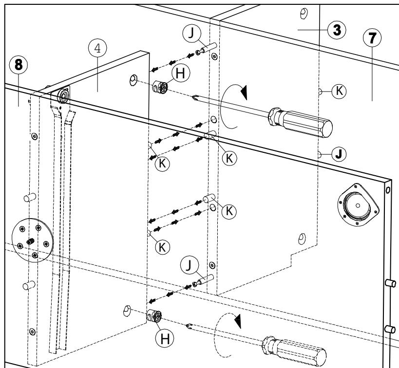
13. Align bottom panel and shelf with end panels as shown. Insert cam locks (G) into top back rail. Insert cam locks (H) into bottom panels and shelf. Tighten with screwdriver.
