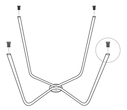
1. Turn base upside down. Insert feet (A) and tap gently with a rubber mallet to fix in place.
