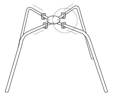
2. Slide spacers (B) on frame close to the metal plate.
