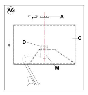
Place the Shade (C) onto the Socket (D), Secure the Shade (C) by tightening the Socket Ring (A) in a clockwise direction until tighten.
