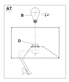
Insert the specified light bulb (B) into the Socket (D). DO
