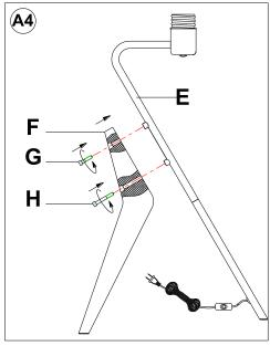
4. Insert the Short Allen Screw (G) and the long Allen Screw (H) into holes of on the Wood Part (F) and Secure the Short Allen Screw (G) and the long Allen Screw (H) on the Upper Curved Tube (E) using a Flat Blade driver until tight.
