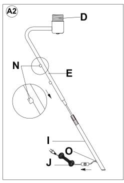
2. Insert the Top Curved Tube (E) into the Lower Tube (I), align short screw tubes (N) with Exit Hole (O) in the same line.
