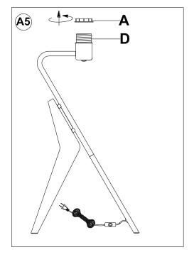
Unscrew Socket Ring (A) from Socket (D) by turning counter-clockwise.
