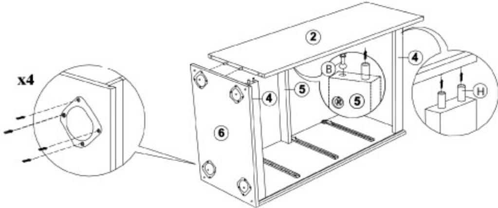
10. Align legs (#8) with bottom and screw in clockwise. Do not overtighten! Slide back panel into groove in back of case. Align top panel and press firmly into place. Turn cam locks 180 degrees until locked. With help stand case upright and do not lean it on the legs they could break.
