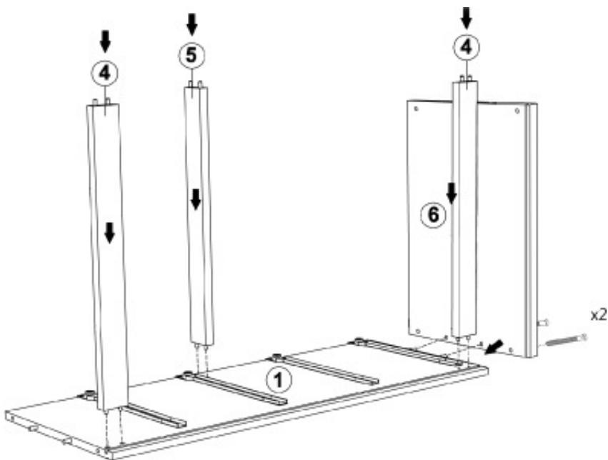
9. With help, align bottom panel (6), and the other end panel (2) over the dowels and cam locks. Press firmly together. Turn the cam locks with the provided hex key 180 degrees until they lock the rails into place. Align the bottom leg supports (L) and insert screws (J). Tighten with phillips-head screwdriver. Do not over tighten!
