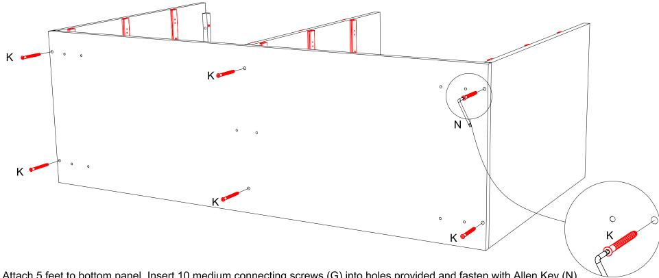
19: Attach 5 feet to bottom panel. Insert 10 medium connecting screws (G) into holes provided and fasten with Allen Key (N). Insert 5 level adjust screws into holes provided.
