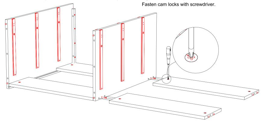
16: Attach right side panel to back panel slats with dowels. Fasten Cam locks with screwdriver.
