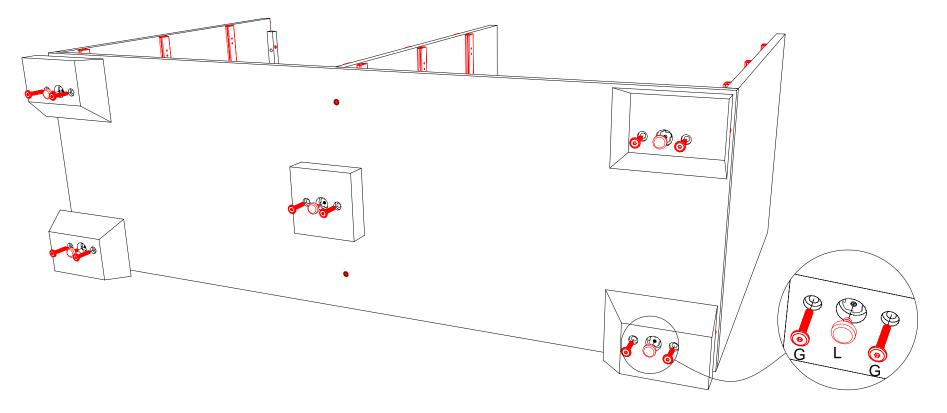
20: Slide long thin back panel into groove on back edge of side panels.
