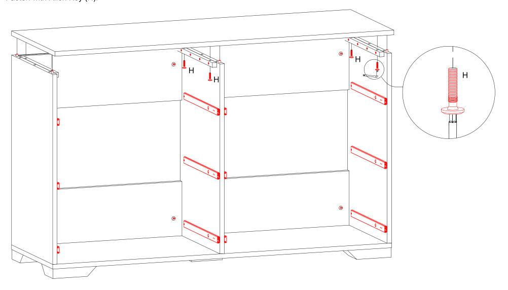
22: Slide 3 left drawers onto drawer rails on left side of dresser. Then slide 3 right drawers onto drawer rails on right side. Insert drawer rail screws (I) into holes provided inside drawer side panels.
