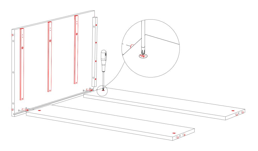
14: Attach back panel slats into holes provided left side of partition panel. Fasten cam locks with screwdriver.
