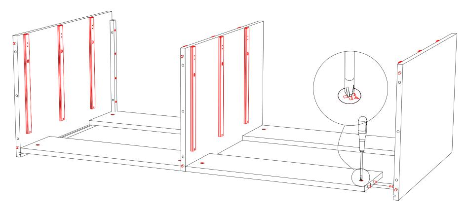
17: Attach bottom panel to left, center and right panels using the 2 dowels previously attached to bottom of each panel.
