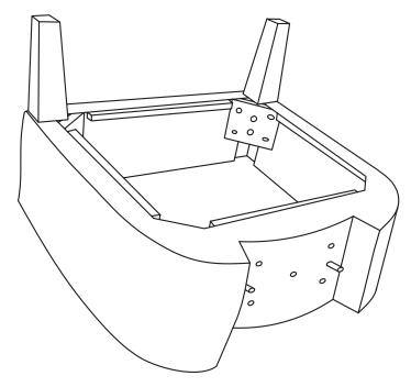
2. Align holes and insert bolt (A), spring washer (C), flat washer (D). Do not tighten completely.
