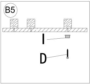
5. Fasten Top Cap (I) to ceiling using Screw(D) into ceiling joist at the marked locations ..Rotate screw clockwise while firmly pressing it into wood by the Phillips head screw driver. If installing through drywall to wood joist, the threaded portion of Screw (D) will drive itself into the drywall and then into the underlying wooden ceiling joist.
