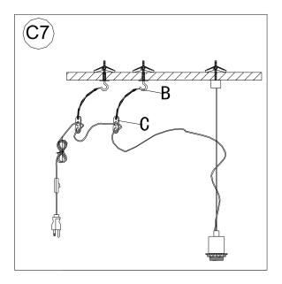
Position the Plastic Clips (C) along the cord so that they align with the installed Toggle Hooks
