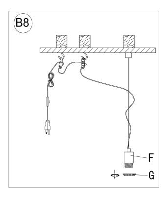
8. Unscrew Socket Ring (G) from Socket (F). Place the shade (not included) onto the Socket (F), and secure the shade by turning the Socket Ring (G) in a clockwise direction until tight. Insert the light bulb into the Socket (F). To avoid the risk of fire, do not exceed the recommended lamp wattage as outlined in page 1.
