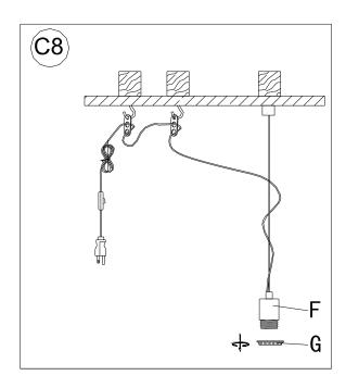
8. Unscrew Socket Ring (G) from Socket (F).Place the shade (not included) onto the Socket (F), and secure the shade by turning the Socket Ring (G) in a clockwise direction until tight. Insert the light bulb into the Socket (F). To avoid the risk of fire, do not exceed the recommended lamp wattage as outlined in page 1.
