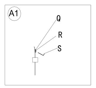
Loosen the two Allen Screws(R) from the Binding Collar (Q) using the Allen Wrench(S).Remove just the short end of the steel cable out of the binding collar hole opening. Slide the Binding collar(Q) along the cable length to the new desired fixture suspension length.
