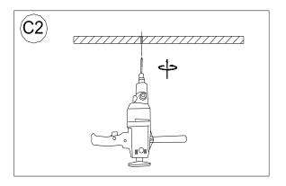
Using the drill with the appropriate size drill bit (just large enough to make hole that will allow passage of the folded Toggle Hooks (B) and Toggle Bolt (C)., drill 1 hole in the ceiling at each of the 3 marked slot locations for the Toggle Hooks (B)and assemblies.
