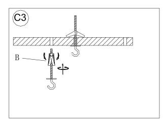
3. Use the Toggle Hooks (B), inserted through each of the 2 ceiling holes, making sure only the Toggle Hooks (B) are fully inserted into the ceiling and toggle wings are open. Rotate each Toggle Hook (B) clockwise until each flat washer on the Toggle Hook (B) is tight against the ceiling.
