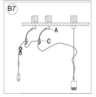
7. Position the Plastic Clips (C) along the cord so that they align with the installed Screw Hooks (A) on the ceiling and carefully fit each Plastic Clip (C) onto each Screw Hooks (A).
