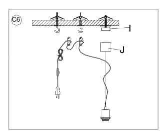
Hang Pendant socket section with the steel cable by screwing Top Cover (J) into ceiling mounted Top Cap(I).
