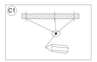
Mark the 2 slot locations of Screw Hooks (B) and the 1 slot locations of Toggle Bolt(C) on ceiling at the desired locations.
