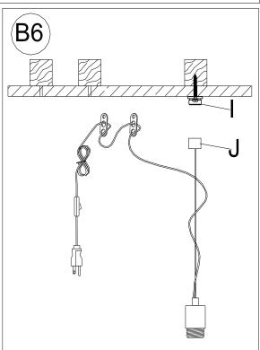
Hang Pendant socket section with the steel cable by screwing Top Cover (J) into ceiling mounted Top Cap(I). Make sure Top Cover (J) is tight to ensure fixture is secure to ceiling.
