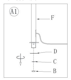
1. Unscrew the Fixing Nut (B), Spring Washer (C) and Flat Washer (D) from the Tube (F) by turning counter-clockwise.
