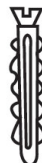
PLASTIC ANCHORS FOR DRY WALL OR PLASTER MOUNTING 1 FOR EACH BRACKET SCREW
