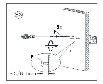
Use the Phillips screwdriver to secure the Wall Screws (F) into each drilled hole. Rotate the Wall Screw (F) clockwise until the screw head is about 3/8 inches from the wall.
