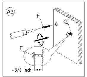
Use a Phillips Screwdriver to insert the Wall Anchors (G) at the marked keyhole locations. Do not "push" or drive the Wall Anchors (G) into the wall, it is designed to bore into the wall like a drill bit. Slowly turn the Wall Anchors (G) clockwise while applying pressure until the flange just touches the wall.
