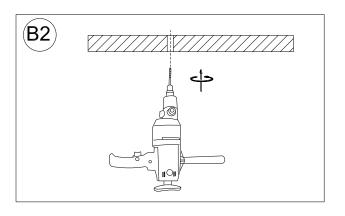
Using the drill with the appropriate size drill bit (just large enough to make hole that will allow passage of the folded Toggle Hooks (B)), drill 1 hole in the ceiling at each of the 2 marked slot locations for the Toggle Hooks (B) assemblies.
