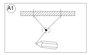
If needed, use a "stud finder" (not included) to locate the ceiling wooden joists and mark their locations on the ceiling using a pencil or a piece of tape. Mark the 2 slot locations of Screw Hooks (A) on ceiling joists at the desired locations
