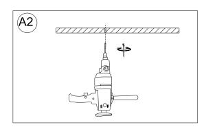
Pre-drill pilot holes at the marked locations. This will make installing the Screw Hooks (A) onto the wall easier.
