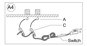
Position the Plastic Clips (C) along the cord so that they align with the installed Screw Hooks (A) on the ceiling and carefully fit each Plastic Clip (C) onto each Screw Hooks (A).
