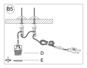
5. Unscrew Socket Ring (E) from Socket (D). Place the shade (not included) onto the Socket (D), and secure the shade by turning the Socket Ring (E) in a clockwise direction until tight. Insert the light bulb into the Socket (D). To avoid the risk of fire, do not exceed the recommended lamp wattage as outlined in page 1.
