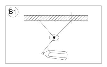
1. Mark the 2 slot locations of Screw Hooks (B) on ceiling at the desired locations.
