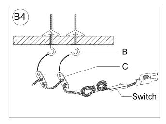
Position the Plastic Clips (C) along the cord so that they align with the installed Toggle Hooks
