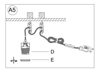
5. Unscrew Socket Ring (E) from Socket (D). Place the shade (not included) onto the Socket (D), and secure the shade by turning the Socket Ring (E) in a clockwise direction until tight. Insert the light bulb into the Socket (D). To avoid the risk of fire, do not exceed the recommended lamp wattage as outlined in page 1.
