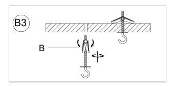
3. Use the Toggle Hooks (B), inserted through each of the 2 ceiling holes, making sure only the Toggle Hooks (B) are fully inserted into the ceiling and toggle wings are open. Rotate each Toggle Hook (B) clockwise until each flat washer on the Toggle Hook (B) is tight against the ceiling.
