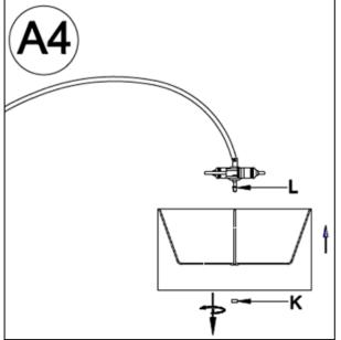
4. Unscrew the Finial (K) from the Threaded Rod (L) by turning counter-clockwise.
