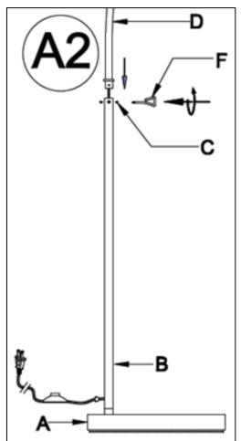
2. Loosen and unscrew 4 Screws (C) from the top end of the Lower Tube (B). Insert bottom end of the Upper Curved Tube (D) into the top end of the Lower Tube (B), making sure the Upper Curved Tube (D) is tilting forwards from the Lamp Base (A). Secure this joint by turning the 4 Screws (C) into the top end sides of the Lower Tube (B) in a clockwise direction using the Screwdriver (F) until tight.
