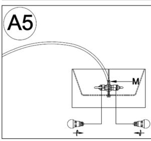
Insert the specified light bulb into the Socket (M). DO NOT EXCEED THE SPECIFIED WATTAGE.
