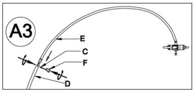
Assemble the Top Curved Tube (E) onto the top end of the installed Upper Curved Tube (D) using the same procedure as outlined in step A2.
