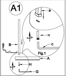
1. With the help of another person, attach the bottom end of the Lower Tube (B) onto the top surface of the Lamp Base (A) as shown in Fig.1, making sure the 2 screw heads on the Lamp Base (A) are aligned and engaged with 2 holes on the bottom of the Lower Tube (B). Secure the Lower Tube (B) onto the Lamp Base (A) by turning the Allen Screw (H) into the bottom threaded hole of the Lower Tube (B) clockwise using Allen Key (G) until tight.
