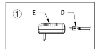
1. Insert the polarity plug (D) into the LED driver (E).
