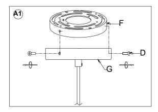
Separate the Mounting Plate (F) from the Canopy (G) by removing the 3 Canopy Screws (D). Do not discard the Canopy Screws (D) as these will be used later.
