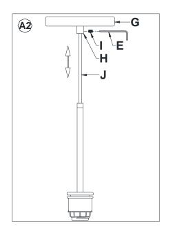
Loosen the Set Screw (I) from the Collar (H) under the Canopy (G) using an Allen Wrench (E) by turning counter-clockwise. Adjust the Power Cord (J) upwards or downwards through the Canopy (G) until a new desired suspension length is determined. Secure the Power Cord (J) in place by tightening the Set Screw (I) onto the Collar (H). Do not over tighten the screw, making sure the Power Cord (J) will not slip downwards with the pendant body.
