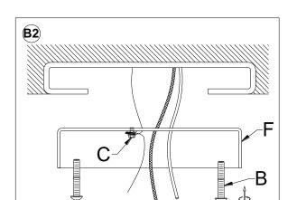
Gently pull existing wire down from the ceiling junction box and allow wires to hang. Attach Mounting Plate (F) to the ceiling outlet box, aligning the slots of the Mounting Plate (F) with the two threaded holes located on the J-Box. Insert and tighten 2 Mounting Screws (B) with a screwdriver.
