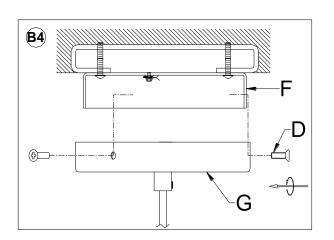
4. With the help of another person to hold the weight of the light fixture, position the Canopy (G) over the Mounting Plate (F), aligning the 3 holes on the Canopy (G) with the 3 holes from the Mounting Plate (F). Insert the 3 Canopy Screws (D) and tighten to secure the Canopy (G) in place.
