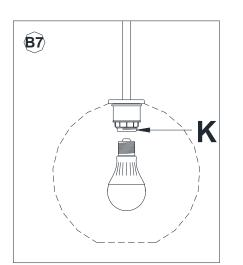
Insert the specified light bulb into the Socket (K). DO NOT EXCEED THE SPECIFIED WATTAGE.
