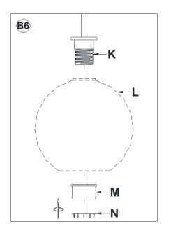
Put the Glass Shade (L) and Spacer (M) onto the Socket (K),secure Glass Shade (L) and Spacer (M) by rotating the Socket Ring (N) in a clockwise direction until tight.Do not over tighten.
