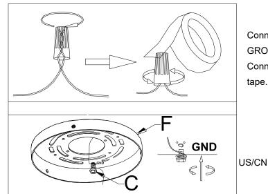
Connect the GROUND FIXTURE WIRE to the GROUND J-BOX WIRE using the Plastic Wire Nut Connector (A) and wrap the connection with electrical tape. Be sure that no wire strands are exposed.
