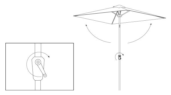
3. To tilt the umbrella top, depress and hold the tilt button while turning the umbrella top to the left or right until it locks in place. IMPORTANT: To avoid damaging your umbrella, be sure to return the umbrella top to its regular upright position before attempting to close it.
