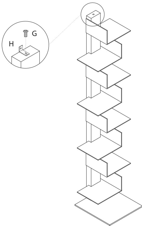
3. Set the bookcase next to the wall. Notice where the angle bracket is in reference to the wall. This is where you must install the anti tip bracket (F). Insert screw (E) thru the anti tip bracket and into the wall (stud mounting is recommended). Once the bracket is secured to the wall you will need to lace the nylon strap (C) thru the anti tip bracket (F) and the angle bracket(G). Pull snugly against the wall.
