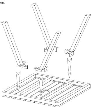
2. Fasten legs to frame using bolts (A) as shown. Put all 16 bolts in loosely before tightening with allen key (B).
